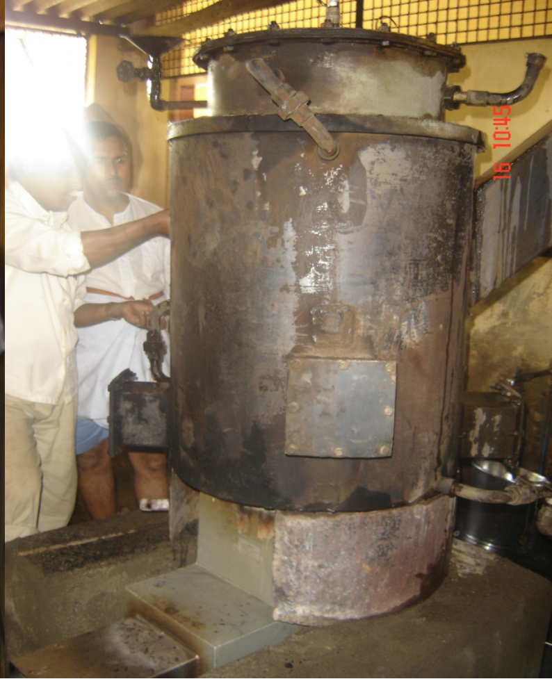
EIGAS stove being used for raising steam for cooking at Ulavi temple (near Karwar)
